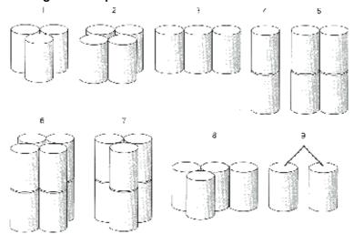
All Yuasa cylindrical cells can be connected together to form higher voltage/capacity packs. Dependant upon quantities required, almost any configuration can be achieved. Pack details are available on request.
