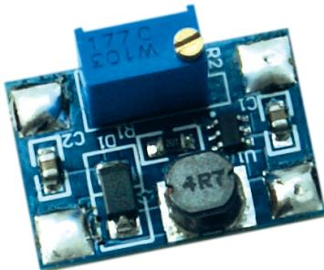
This is a high-performance switching boost and buck module with 1.1A current.
