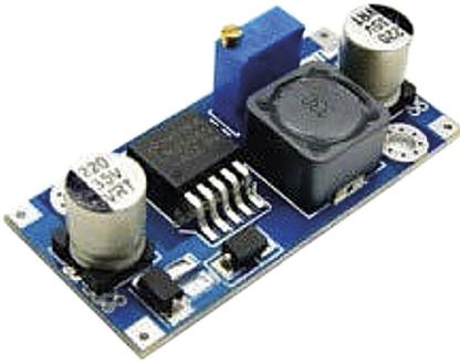
This is a high-performance switching buck module with 2A current.
