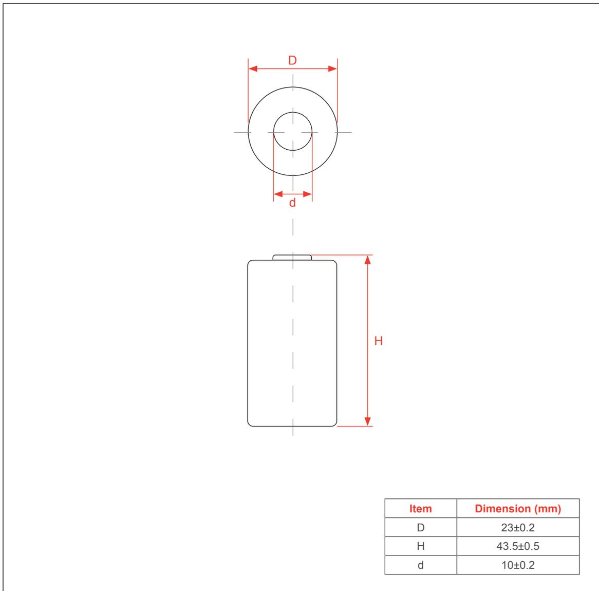
NH4100SCBFRP • Nickel metal hydride battery
