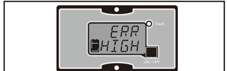
6. Battery high volt protection.
