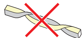
(as the picture shows) please do not twist the strip, or it will be damaged.
