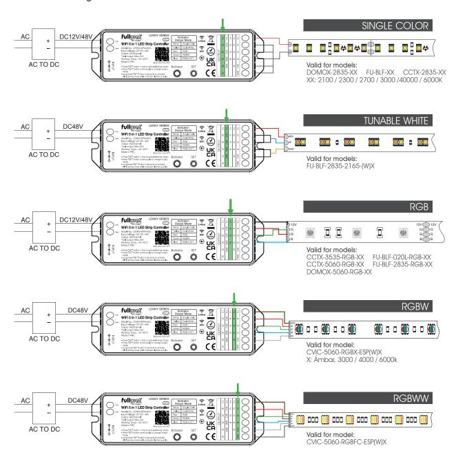
"Switch" button can be used to indicate which type of product is being managed. To do so, press the "Switch" or "SET" button with a short touch until color from "indicator light" is required one.
