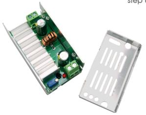
This is a high-performance switching boost module with 7A current
