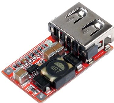
This is a high-performance switching buck module with 2A current.
