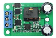
This is a high-performance switching buck module with 5A current.
