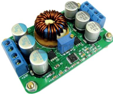
This is a high-performance switching buck module with 6A current.
