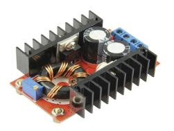
This is a high-performance switching boost module with 6A current.
