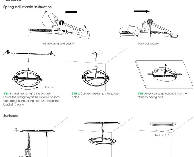
STEP 2 Connect the lamp's the power
