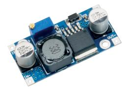
This is a high-performance switching buck module with 0.5A current.
