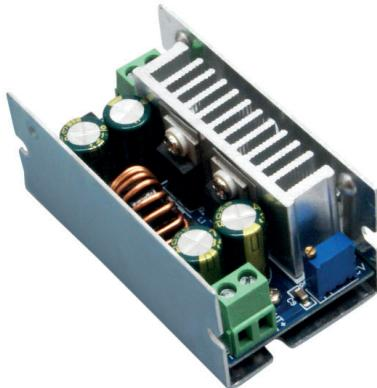
This is a high-performance switching buck module with 7.5A current.
