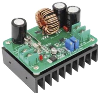
This is a high-performance switching boost module with 10A current.
