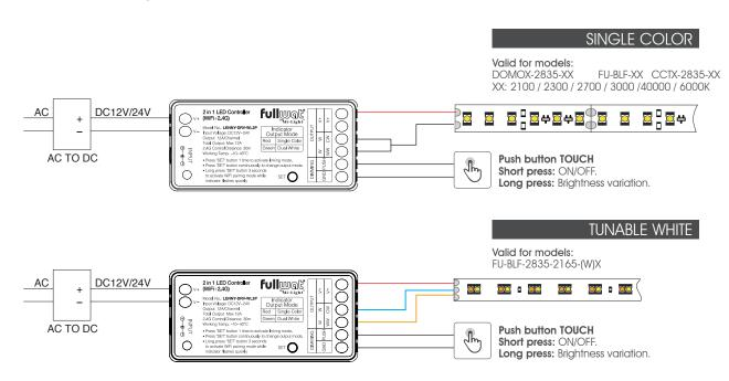
Press "SET" continuously to switch between single color and tunable white mode.
