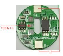
P+ = B+ = Charge+/Discharge+ P- = Charge-/Discharge-
