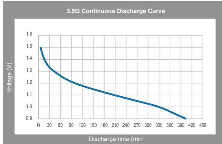
b. Load resistance: 3.9Ω Discharge pattern: 1h/day End Voltage: 1.0V Temperature: 20°C±2°C
